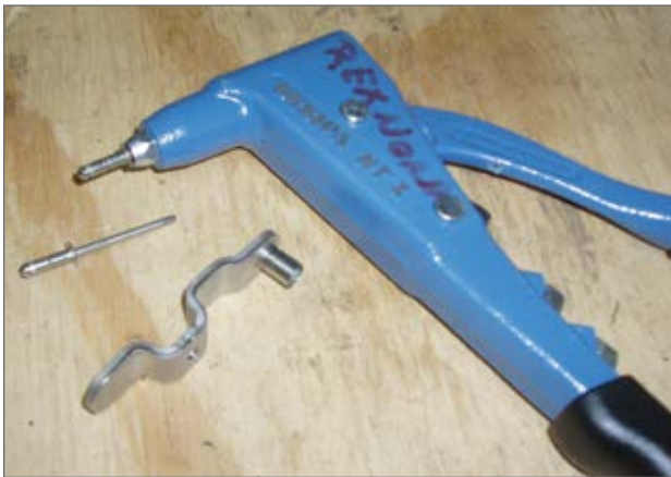
9200 chain rivet tool, clip and stainless steel rivet
