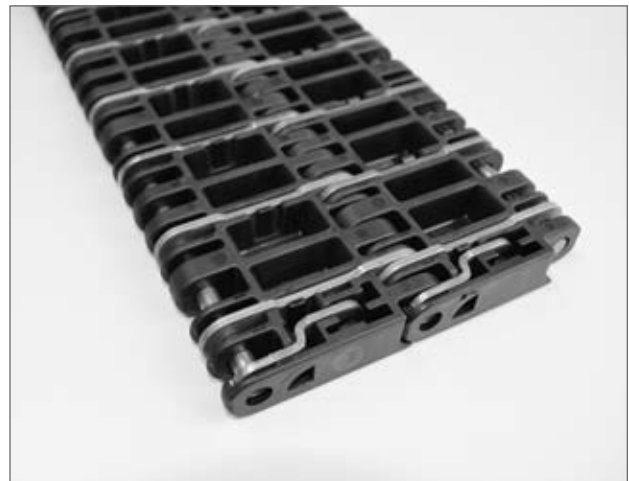
Assembly — Reinsert pin and rotate pin retention to full closed position until you can feel and hear 'click'
