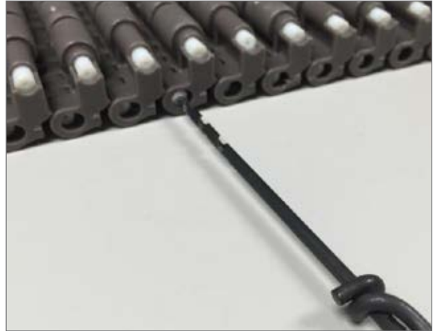
Disassembly — Insert a pin puller into end of pin from either side of chain
